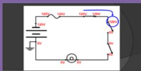
When we shut the first switch, we see that the last point of potential is now directly upstream of the second switch.
