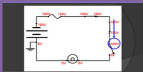
With each successive switch, we move the last point of potential toward the load until all of the switches are closed.
