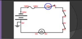
During normal operation with the switches open, these are the voltages you will see. Since the first switch is an intentional break in the circuit, the last point of potential is directly upstream of that switch.
