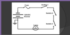
Consider this simple circuit, which contains a 120VDC Battery, a single fuse, three SPST switches, and a lamp.
