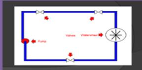
Recall from basic electricity I that voltage is analogous to pressure in a fluid system. In this fluid system, we have a pump for our flow source, a water wheel for our load, and three valves that will serve as control devices.
